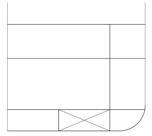
Fig. 7 Heeling tank in double bottom
