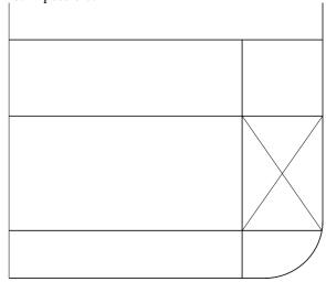
Fig. 4 Heeling tank one 'tween deck high
